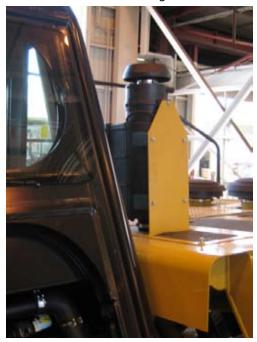
Below: The flex hose goes from the unit to a hole cut into the low-pressure side of the HVAC plenum. The original air intake has been sealed off.
